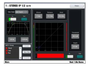
The noise gate provides a full set of controls and signal metering as you would find on a top grade outboard processor. A self keyed side chain filter may be switched in or out. Use the controls or screen to set the threshold (a signal meter displays under the control to help you set this quickly), depth (how much the gate attenuates), hold time (how long the gate remains open after the signal drops below the threshold), and dynamics. A screen histogram displays the gate activity over time.
